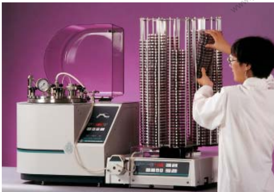
Petri dishes can be aseptically filled and stacked in the PourMatic (right), an automated dish-filling system.
